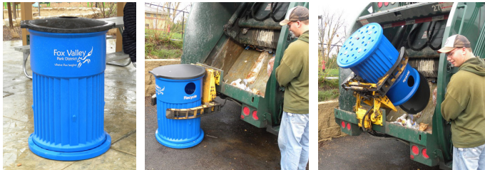
Power lift images show how bin rib/lug configuration facilitates automated handling.
